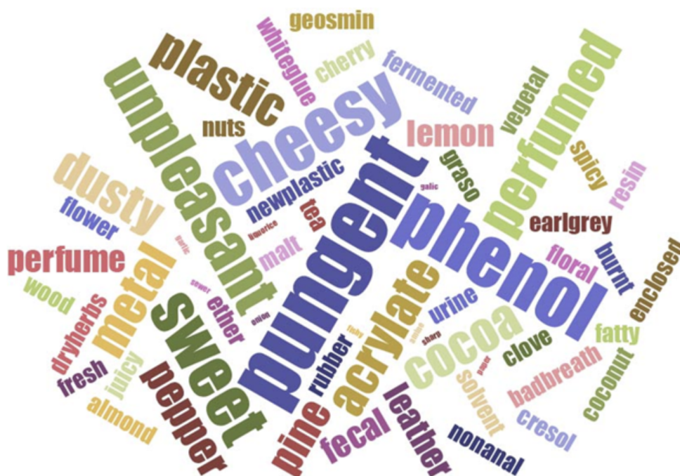
Figure 18: Odour profile of historic car interior Rover P5B smell reflecting GC-O analysis.
